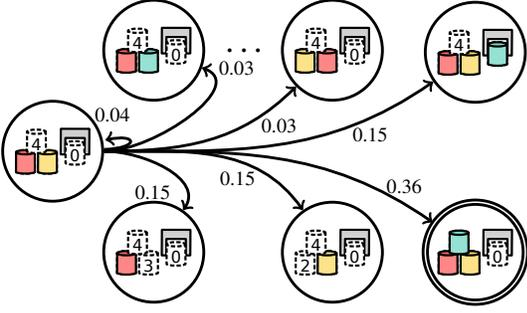
Fig. 6: Example portion of the MDP for our pick-and-place domain with both human and robot actions. The robot action is “pick\_blue.” There is a 36% chance that this succeeds, a 4% chance that it is attempted without interruption but fails. The remaining states are the results of human actions.
