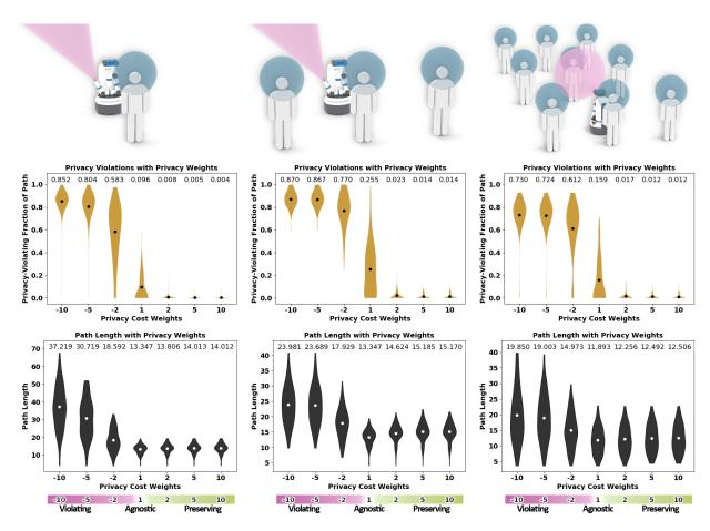
Fig. 3. (Top) A Fetch robot (with camera visibility cone in pink) controlling either the **arm+torso** with a hand camera (left, middle) or the **base+head** with a head camera (right). (From left to right) 1, 3, and 9 privacy regions (blue spheres) overlaid on humans in the workspace. Violin plots (with mean markers) for 100 random runs with the privacy violating fraction (middle) and path lengths (bottom) for different privacy weights. Mean values are given at the top.
