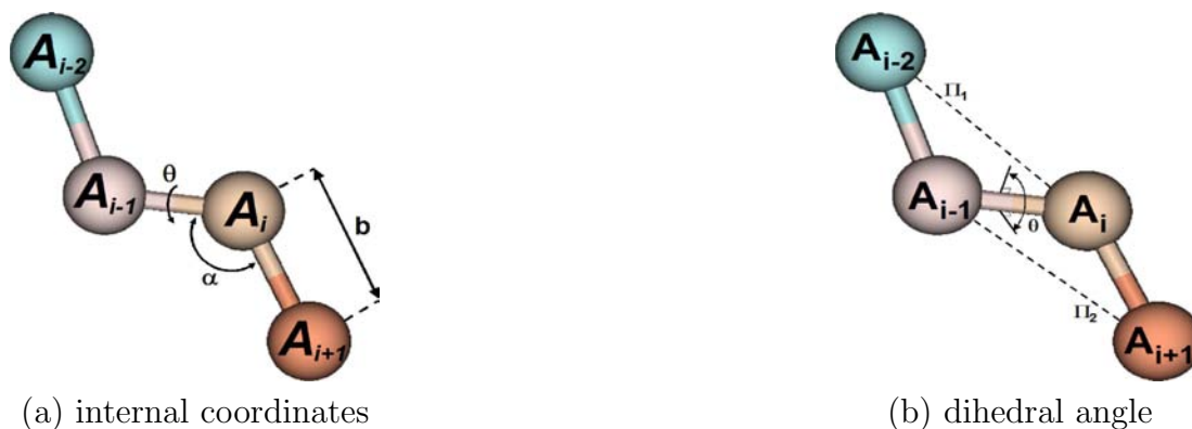
Fig. 2.3: (a) Illustration of internal coordinates, where b refers to bond length, \alpha to bond angle, and \theta to dihedral angle. (b) Rotation by the dihedral on the second bond induces spatial motion of the fourth atom and any consecutive atoms down the polypeptide chain. Figures are generated with MOLMOL [KBW96].
