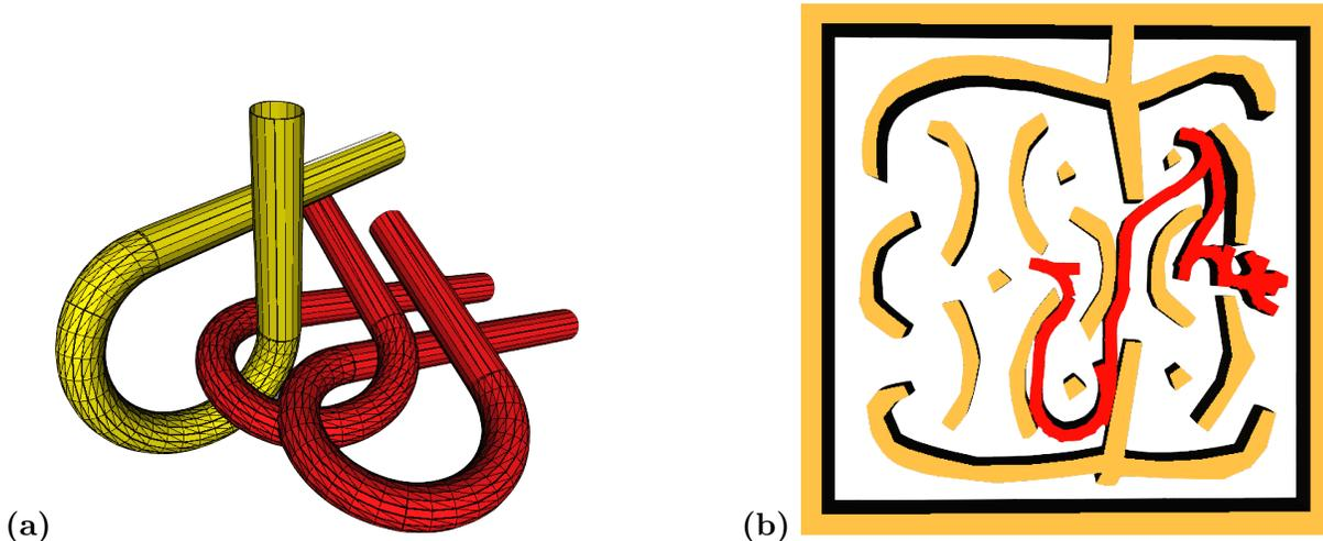
Figure 1. Two sample motion planning problems. (a) The alpha puzzle: the red alpha shape needs to be moved from its initial interlocked pose to a pose where it is separated from the yellow alpha shape. Here the yellow alpha shape can be regarded as an obstacle. (b) A solution path for a car-like robot in a maze. The “car” (modeled by a red box) cannot move sideways and has a bounded turning radius.
