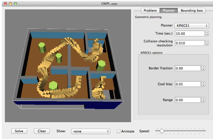
Figure 2. The OMPL.app GUI showing a path for an L-shaped robot in an office-like environment with two floors and a staircase joining them.
