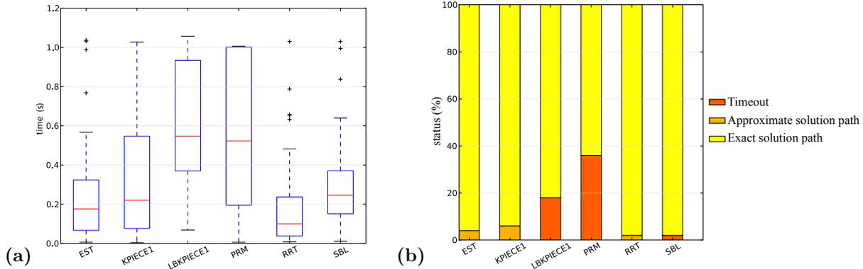
Figure 3. **Sample out of OMPL’s benchmarking tool.** Both plots are based on 50 runs of each algorithm. **(a)** A box plot of run time for different algorithms whose names are indicated on the x-axis. **(b)** A stacked bar chart of planner status distributions. Other possible status values that did not occur in this case include *crash* and *invalid* start/goal state, which can provide useful diagnostic information.
