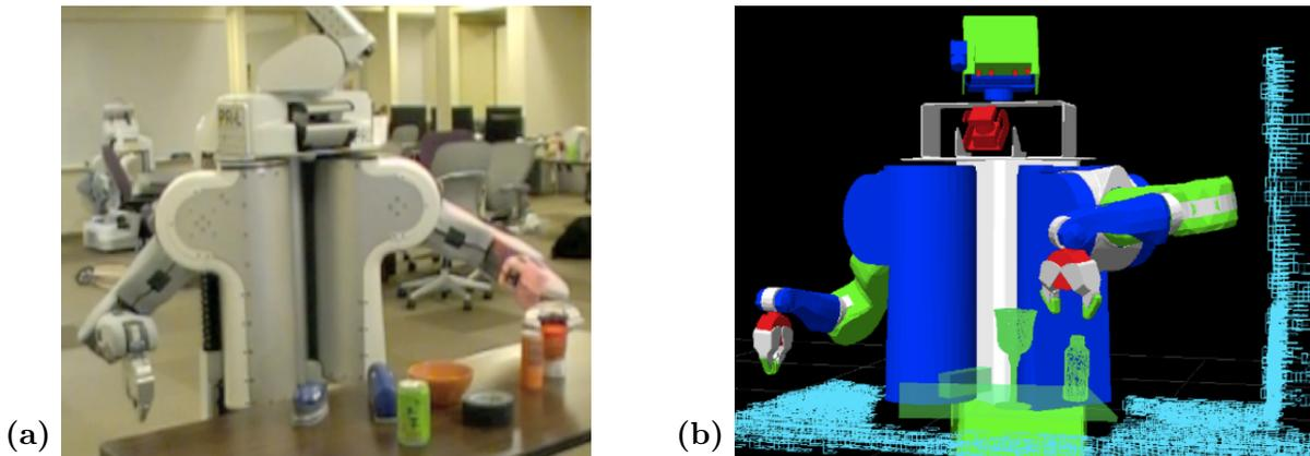
Figure 7. (a) A PR2 robot from Willow Garage performing manipulation tasks using OMPL. (b) The sensed model of the world used for planning.
