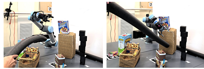
Fig. 9: Reactive planning with moving obstacles: our UR5 robot successfully performs a “pick, place, and reset” loop with our FLASK-RRTConnect planner without colliding with any of the static or moving obstacles. The obstacles are observed by an overhead Intel Realsense camera.
