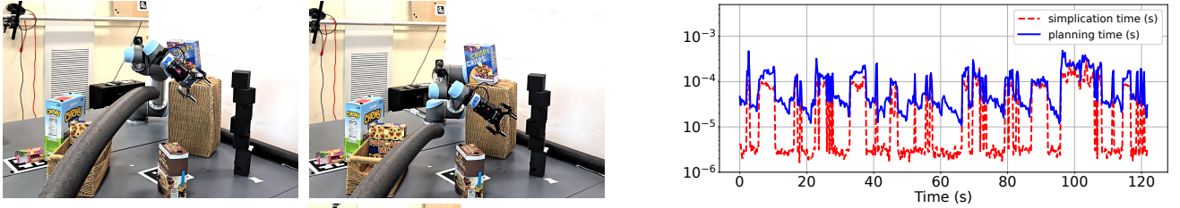
Fig. 10: Planning and simplification time in our “pick, place, and reset” loop: our planner takes \sim 90\mu s and \sim 40\mu s for planning and simplification, respectively, illustrating the reactivity of our approach for real-time applications.
