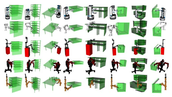
Fig. 6. Representative problems from the 40 different prefabricated datasets provided with MOTIONBENCHMAKER. There are 8 nominal scenes and 5 robots, which create the 40 datasets, each consisting of 100 different problems.
