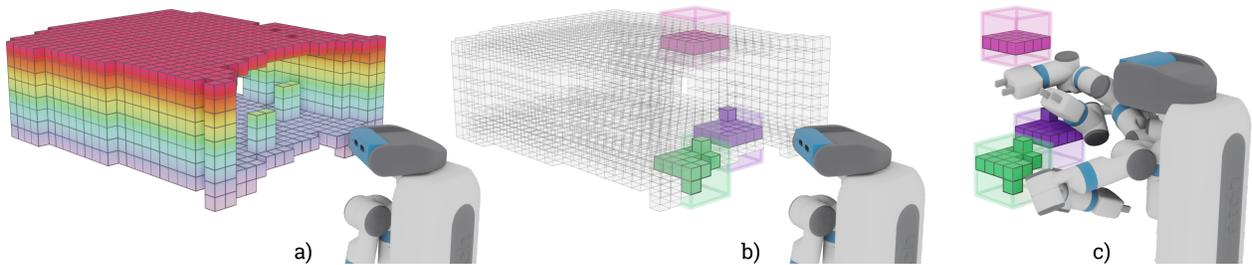
Fig. 3. An example of FLAME, our experience-based planning framework that uses a decomposition of an octomap [8] workspace gathered from sensing data. **a)** The global workspace as an octomap. **b)** Three local primitives (highlighted in color) from the FLAME decomposition. Local primitives are  $4 \times 4 \times 4$  occupancy grids derived from the global octomap. **c)** A set of superimposed samples drawn from the local samplers.
