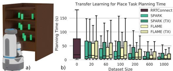
Fig. 6. **a)** The “Large Shelf” environment with a “pick” and “place” task. Three stacked shelves are generated similar to the “Small Shelf” environment (Fig. 4a). The stacked shelves vary relative to the robot in angular placement  $\pm 90^\circ$  and position of X- and Y-coordinates by  $\pm 10\text{cm}$ . **b)** Plot of average planning time (including retrieval) versus the size of the dataset, tested on 200 sampled environments with a timeout of 300 seconds.
