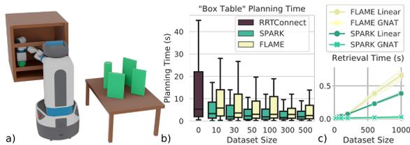
Fig. 5. **a)** The “Box Table” environment with a “place” task. The table and box vary relative to the robot in angular placement  $\pm 30^\circ$  and position of X- and Y-coordinates by  $\pm 10\text{cm}$ . **b)** Plot of average planning time (including retrieval) versus the size of the dataset, tested on 100 sampled environments with a timeout of 120 seconds. **c)** Mean local primitive retrieval time versus the size of the dataset.
