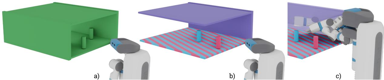
Fig. 2. An example of SPARK, our experience-based planning framework that decomposes the workspace into pairs of known obstacles. **a)** The global workspace, composed of a set of boxes and cylinders. **b)** Three local primitives (different pairs are shown with blue, magenta, pink color) from the SPARK decomposition. Note that the bottom of the shelf is shared between two primitives. **c)** A set of superimposed samples drawn from the local samplers.
