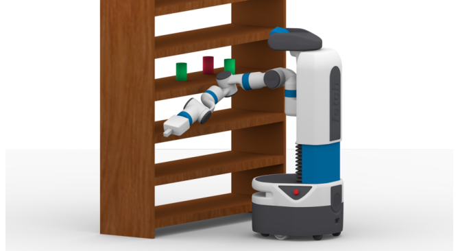
Fig. 1: The task of grasping the red can without removing the green cans is very challenging for traditional methods. The proposed approach efficiently solves it by using prior experiences to guide the search.
