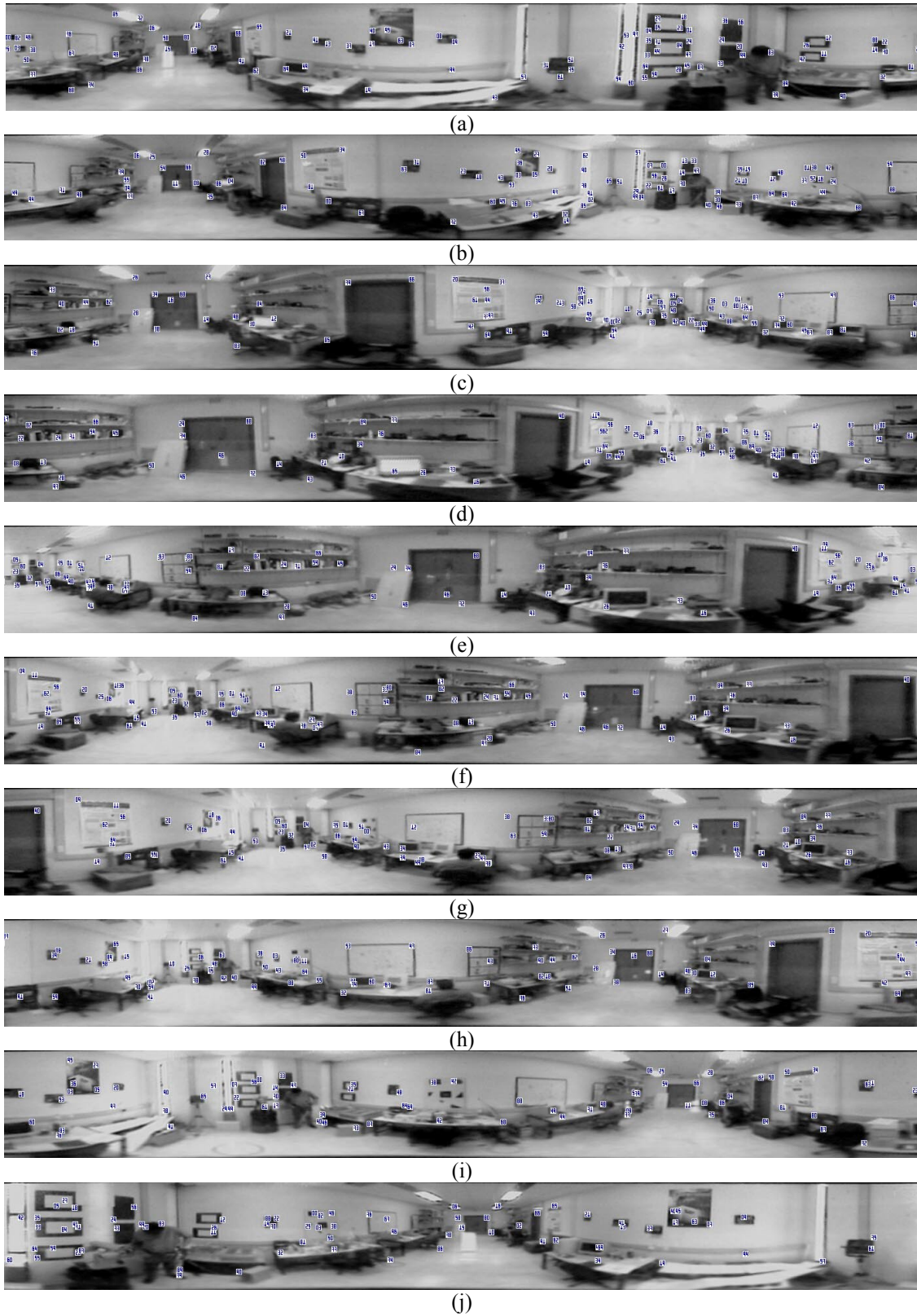
Figure 6: Panoramic images and corner tracking as the robot departs from and returns back to the home position
