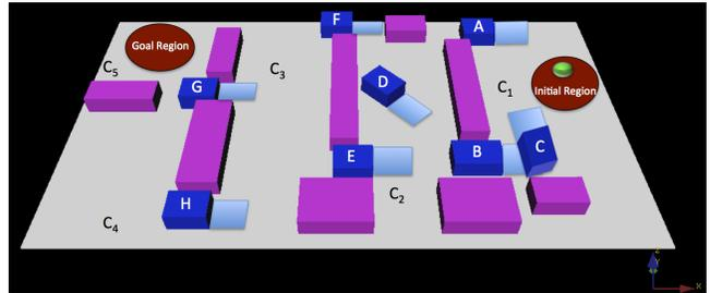
Fig. 1: Manipulation problem: the robot (green sphere) has to move from the initial to the goal region among fixed and manipulatable obstacles (labeled according to their weight in a decreasing order). Workspace regions are labeled with the names of the associated configuration space disconnected regions.
